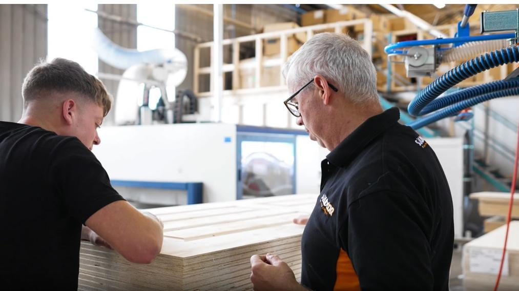
All Solidcor doors have a solid timber core, so the doors are classed as a timber-based door even though they are faced with u-PVC skin for ease of maintenance.
